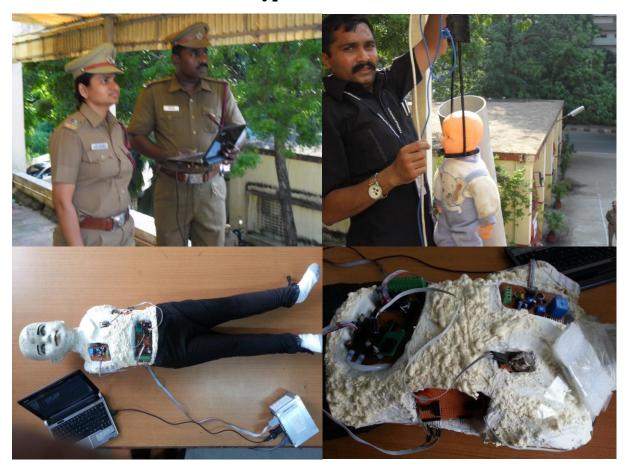
2012 prototype of child model with sensor unit to analyse the gaseous substrate and the deep well analyses was developed and tested to help the paramedical team after rescue operation
